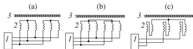
**Fig. 1.** Connection diagram of modules of linear induction. 1—Voltage inverter. 2—Inductor modules. 3—Secondary element.
