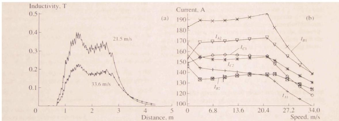
**Fig. 4.** Parallel connection of modules with common neutral: (a) is the induction distribution along the gapping at a speed of 21.5 and 33.6 m/s and (b) is the phase currents amplitude variation in the velocity function.
