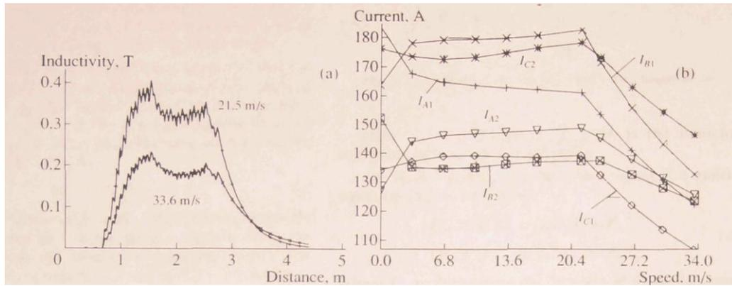
**Fig. 3.** Parallel connection of modules with insulated neutral: (a) is the induction distribution along the gapping at a speed of 21.5 and 33.6 m/s and (b) is the phase currents amplitude variation in the velocity function.
