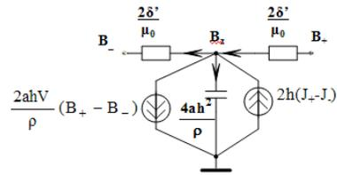
Fig. 2. Equivalent circuit of a field area with a length of  $2h$ .
